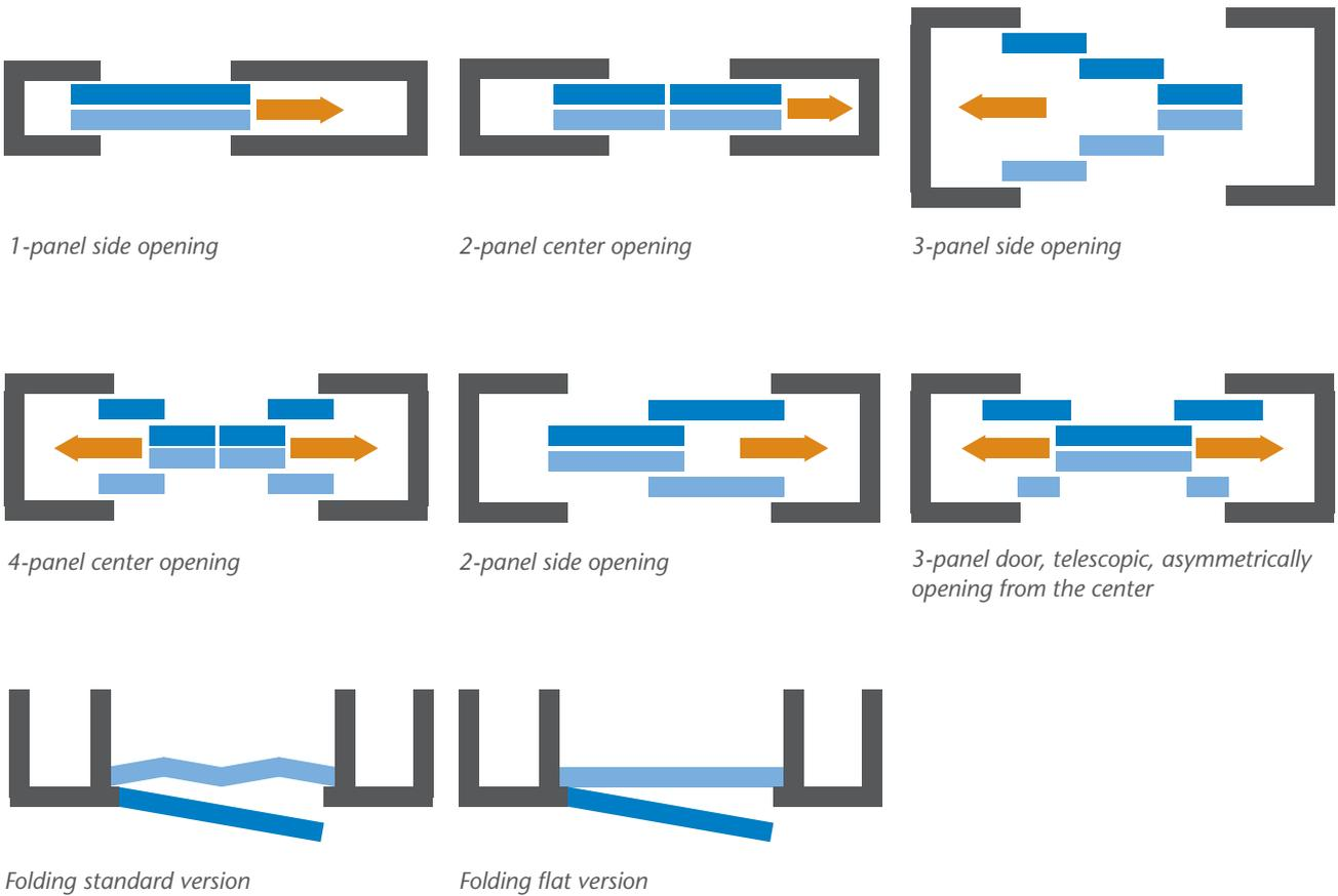
You can select the door opening solution based on the free opening required and the space available.
